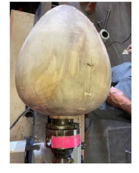
piece attached to lathe using small router to cut area for bow tie. Insert same then sand down
